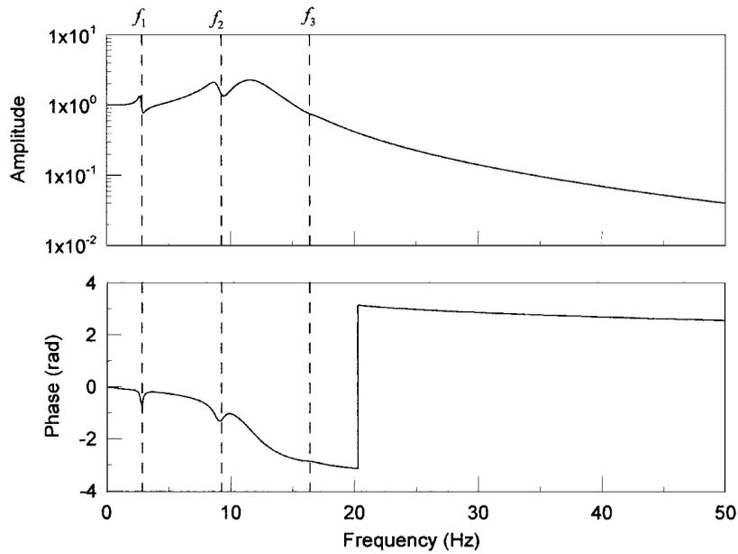
Figure 10. Total transfer function of NEES@UCLA linear shaker in the example building,  $H_{CSI}(s)$ .
