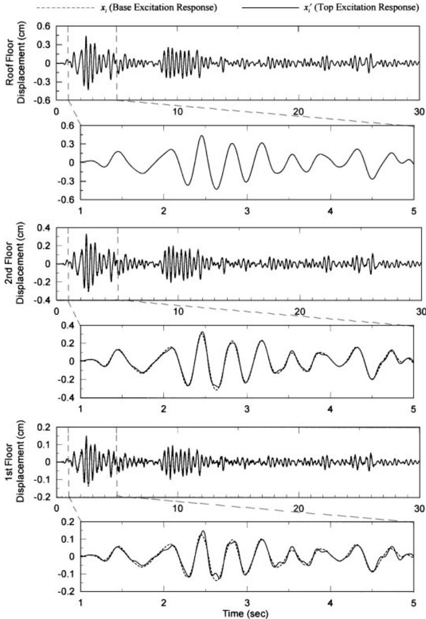
Figure 5. Comparison of base and top excitation responses calculated with the transfer function method (match enforced at Floor 3 using  $T_3(s)$ ).
