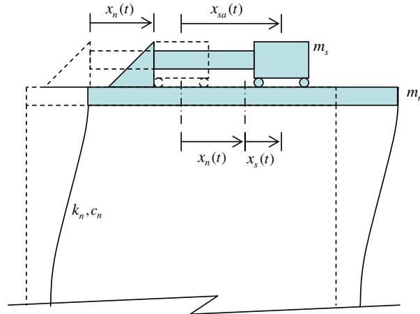
Figure 2. Definition of displacement quantities for linear shaker on a test structure.
