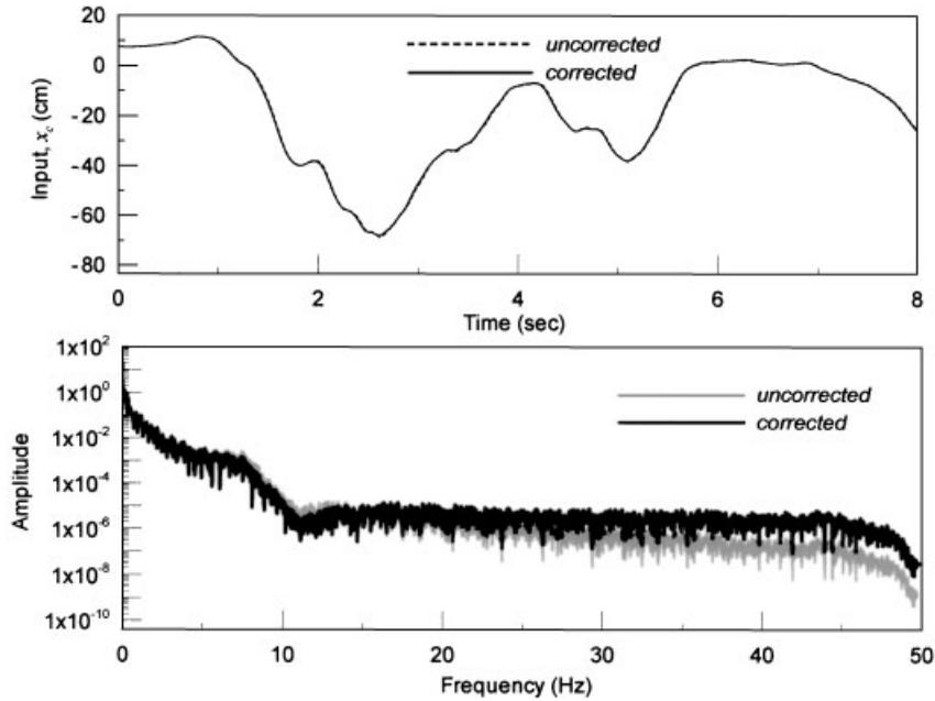
Figure 12. Comparison of shaker input displacement derived using transfer function method with and without correction for CSI effects ( $T_3$  and  $T'_3$  for 1940 El Centro control earthquake ground motion).
