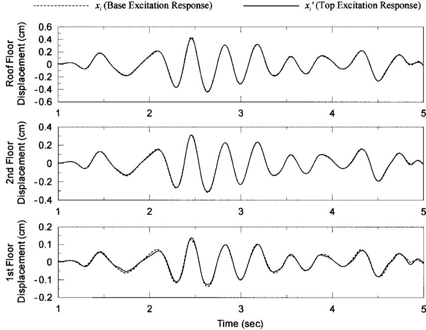
Figure 8. Comparison of base and top excitation displacement responses using the least squares method.
