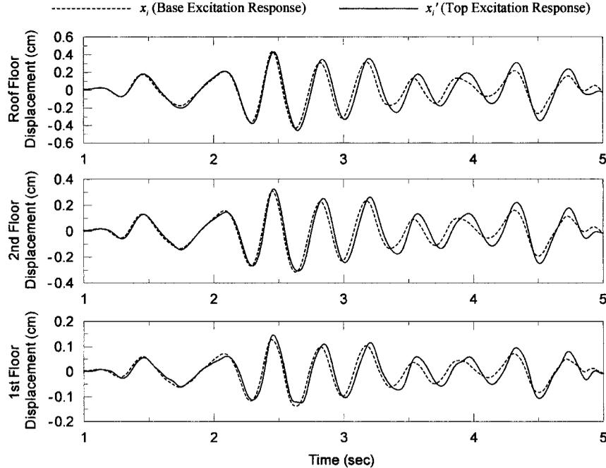
Figure 15. Building displacement response from uncorrected input using least squares method compared with desired response (for base excitation), El Centro 1940.
