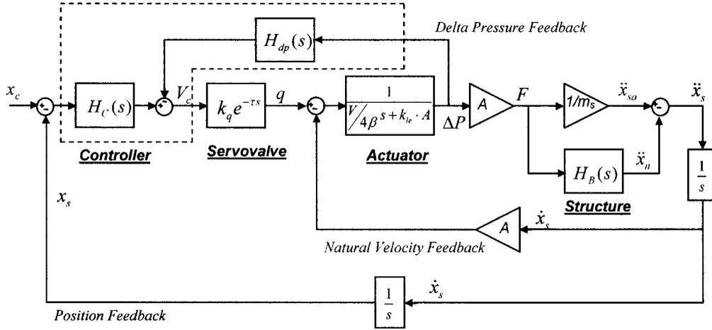
Figure 9. Block diagram model of shaker–structure system.
