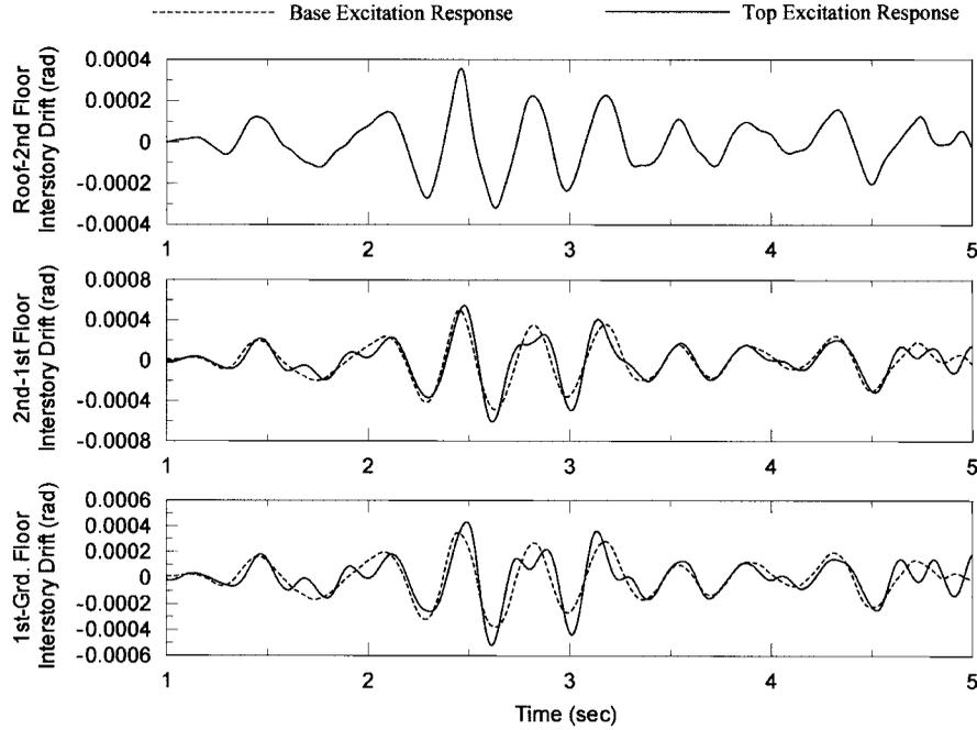
Figure 7. Comparison of base and top excitation interstory drift responses calculated with the transfer function method (enforced match of  $\Delta_{32}$  using  $T_{32}(s)$ ).
