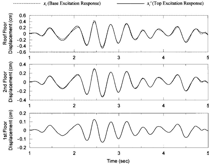
Figure 6. Comparison of base and top excitation responses calculated with the transfer function method (match enforced at Floor 1 using  $T_1(s)$ ).
