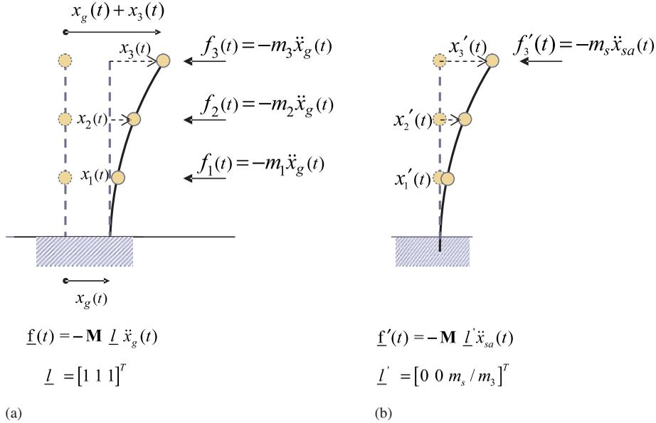
Figure 1. Comparison of effective force distributions for earthquake excitation and shaker excitation; (a) base excitation; and (b) top excitation.
