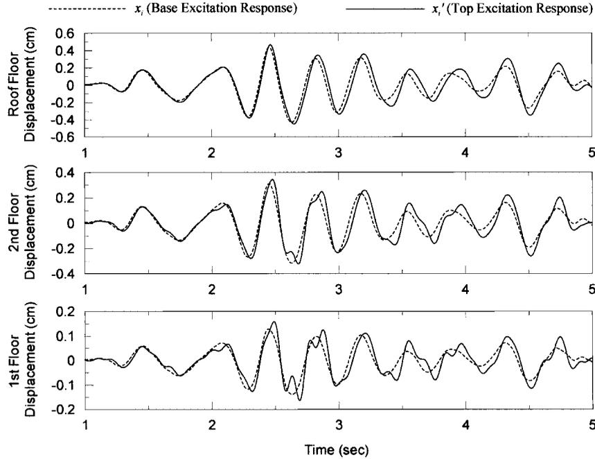
Figure 14. Building displacement response from uncorrected (for CSI effects) input using transfer function method for match of roof floor displacement compared with desired response (for base excitation), El Centro 1940.
