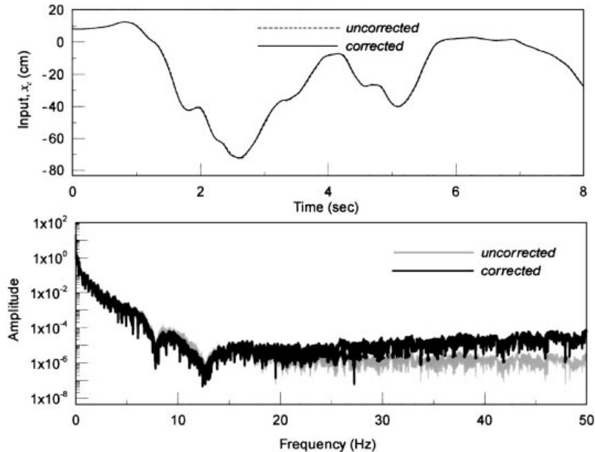
Figure 13. Comparison of shaker input displacement derived using least squares method with and without correction for CSI effects (1940 El Centro control earthquake ground motion).
