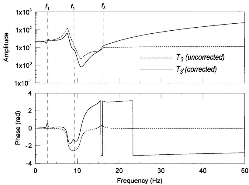
Figure 11. Comparison of amplitude and phase spectra of filter that includes CSI effects ( $T'_3$ ) and that neglects CSI effects ( $T_3$ ), transfer function method.
