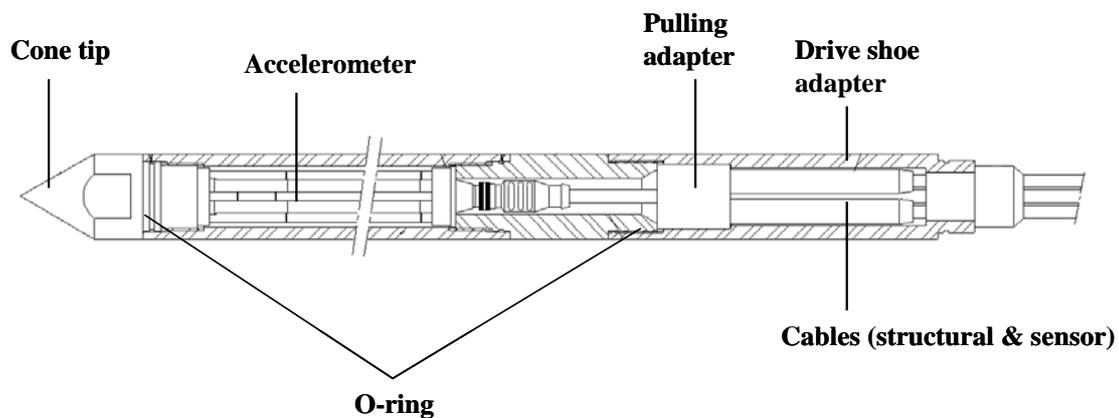
Figure 3. Schematic of the UCLA NEES Retrievable Subsurface Accelerometer
