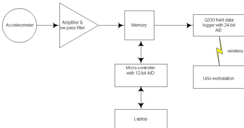
Figure 2. Block diagram of RSA circuit
