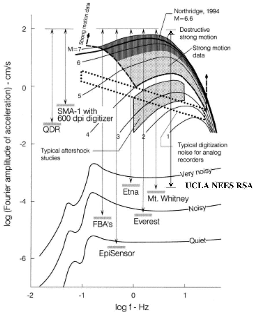
Figure 1. Comparison of Fourier spectrum amplitudes of selected accelerometers (after Trifunac and Todorovska, 2001)
