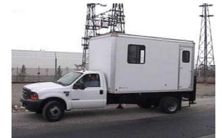
Cone Penetration Testing Truck
